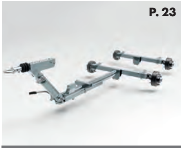
CHASSIS BASIC - TANDEM AXLE BRAKED WITH HEIGHT ADJUSTABLE DRAWBAR
