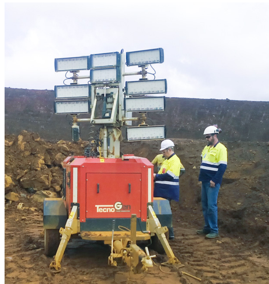
Approved Off – Road LED Lighting Tower, Gross Weight 2,5 Ton
