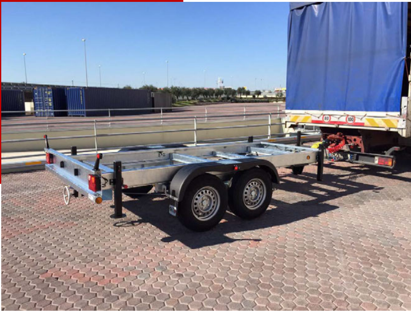
Approved On – Road Trailer, Gross Weight 3,5 Ton, Air Brake System, twin axle, Adjustable Height Drawbar
