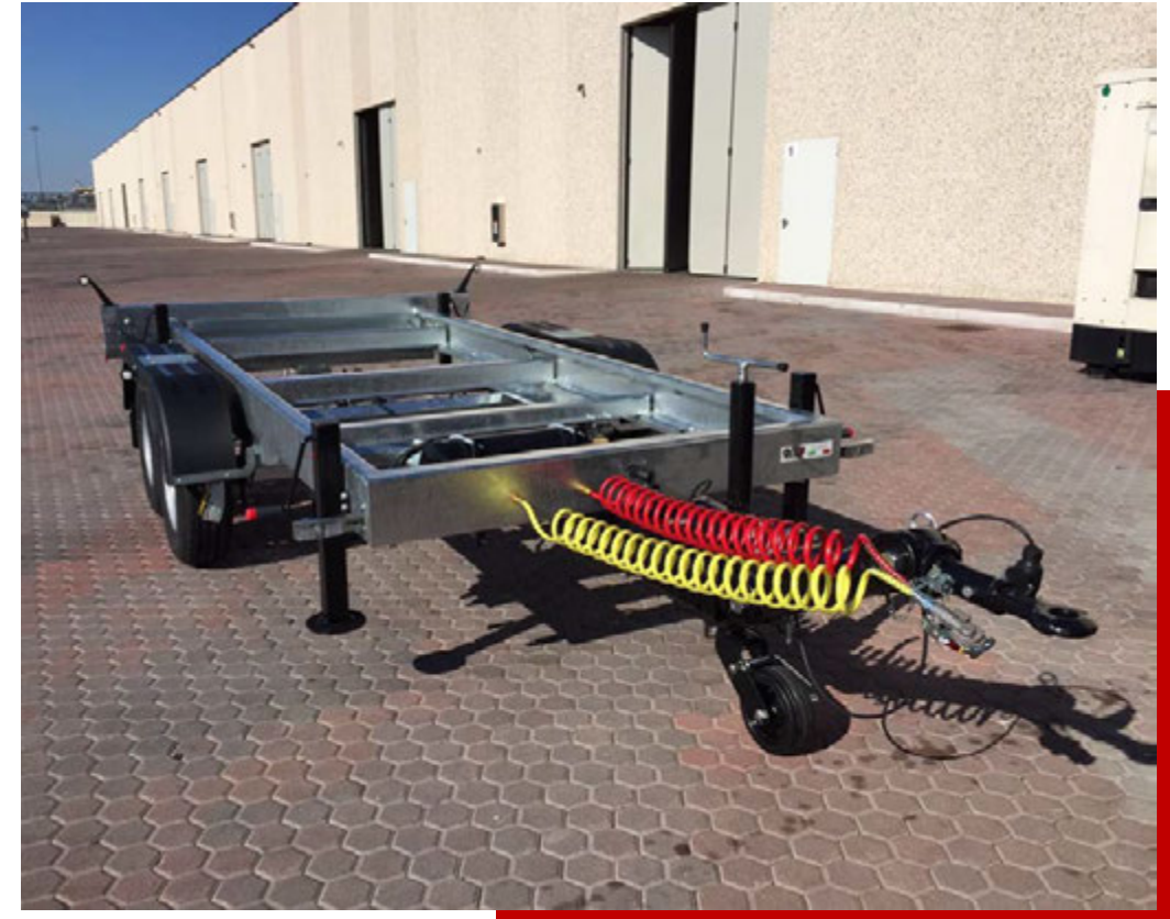
Approved On – Road Trailer, Gross Weight 3,5 Ton, Air Brake System, twin axle, Adjustable Height Drawbar
